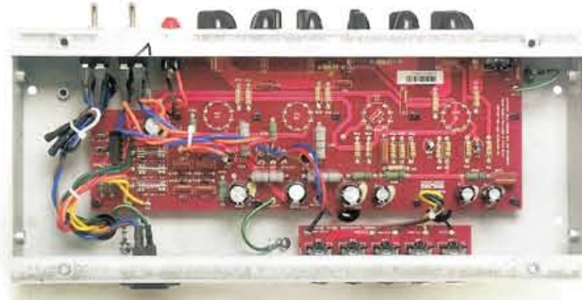
The BH15H's tidy interior features a heavy-duty PC board with thick copper traces. Most of the components are board mounted, including the pots, jacks, and tube sockets.
